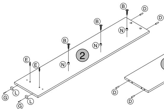
FIXE OS PINOS MINIFIX (E) E AS CAVILHAS (D) NAS LATERAIS E DIVISÓRIA. FIXE AS SAPATAS (L) COM PREGOS (G) E A PARADA DA PORTA (N) COM PARAFUSOS (B)
