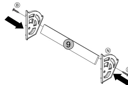
FIXE O APOIO SAPATEIRA NO SISTEMA PIVOTANTE (N) COM PARAFUSOS (B)
