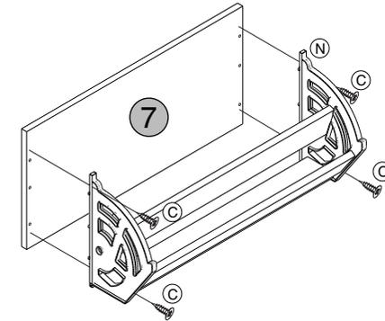
FIXE A MONTAGEM DO SISTEMA PIVOTANTE (N) NA FRENTE
