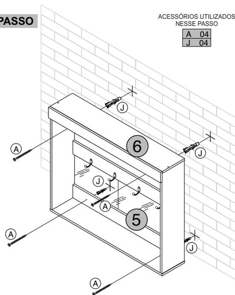
FIXE O PRODUTO NA PAREDE USANDO BUCHAS (J) E PARAFUSOS (A)
