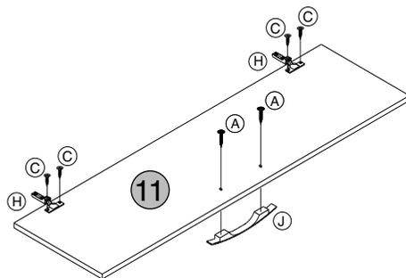
FIXE OS PUXADORES (J) COM PARAFUSOS (A) NA PORTA. FIXAR AS DOBRADIÇAS (H) COM PARAFUSOS (C) NA PORTA
