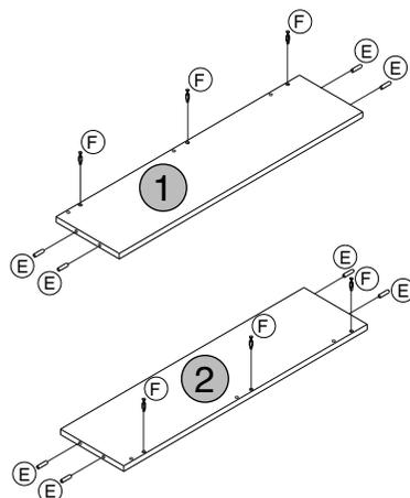
FIXE AS CAVILHAS (E) NAS TRAVESSAS. FIXE OS GANCHOS (H) NA TRAVESSA SUPERIOR E NA TRAVESSA CENTRAL COM PARAFUSOS (C)
