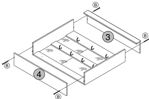
FIXE A BASE E O TAMPO NAS LATERAIS COM PARAFUSOS (B)
